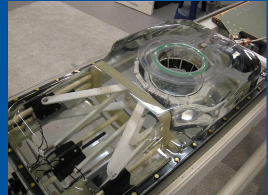
Water box with transducer and motors
